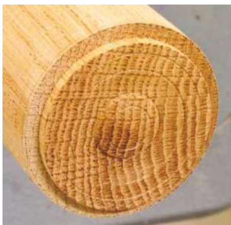
▲ Pic.16 The lid section is now mounted in another chuck. Clean off the bottom of the lid – putting detail on it proves that you have turned it, adding a little class to the piece
